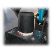
Note: If using a Bronze type bushing, you will have to modify the height of SE60 bushing. The bronze bushings are made to run with a pre-load style arm, therefore the deviates from factory dimensions. We have seen anywhere from .060" to .090" removed to attain proper resistance.
