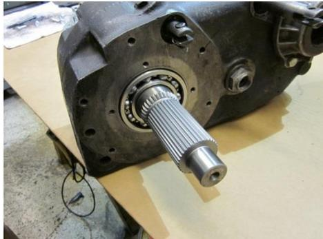
Now to the Magnum housing. Remove the two bolts that retain the shifter housing and remove the shifter housing. There are six socket head cap screws in the front face of the Magnum box that hold the two case halves together, remove them and separate the two case halves.
