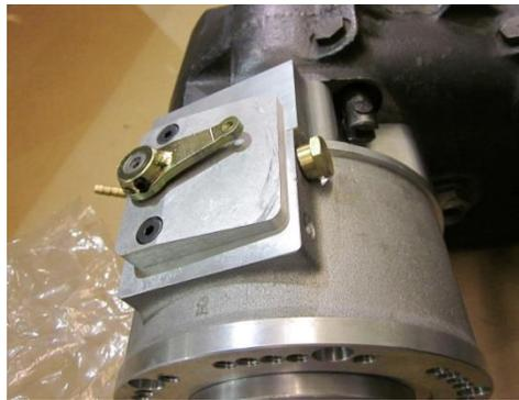
You can fill the Magnum box from either the shifter housing opening or the fill plug location, capacity is 1-1/2 pints (or  $\frac{3}{4}$  of a quart) of automatic transmission fluid or gear oil (80W-90 etc). To visually inspect fluid level, install a clear vinyl sight tube between a barb fitting in the drain hole and a "T" fitting in the vent location or a barb fitting in the fill hole.
