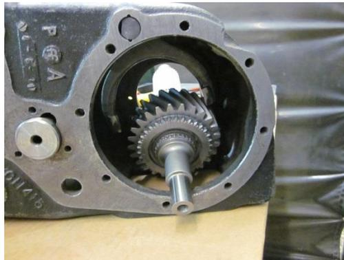
Install the clutch ring onto the shift fork, the shift rail may need to be manipulated for clearance.
