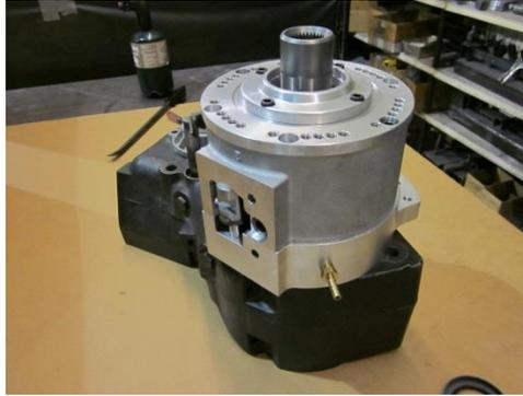
Install the shifter housing using the two supplied bolts, seal the shifter housing with silicone sealant.
