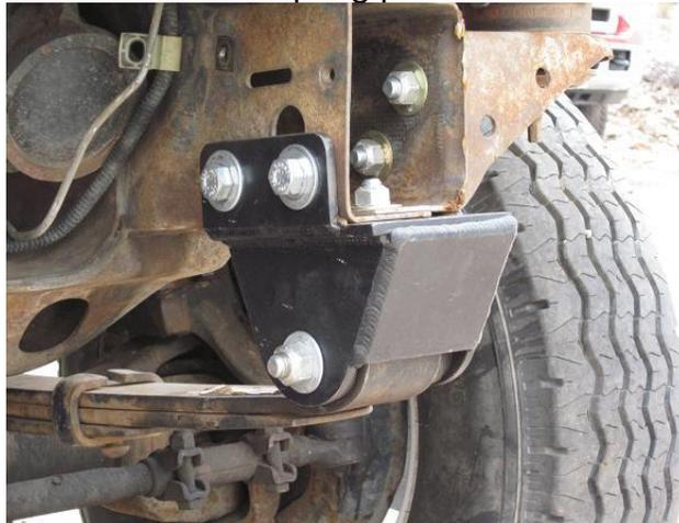
Position rear hanger such that the distance from the main eye centerline to the upper shackle bolt is 51". You will be using the rearward most shackle bolt
