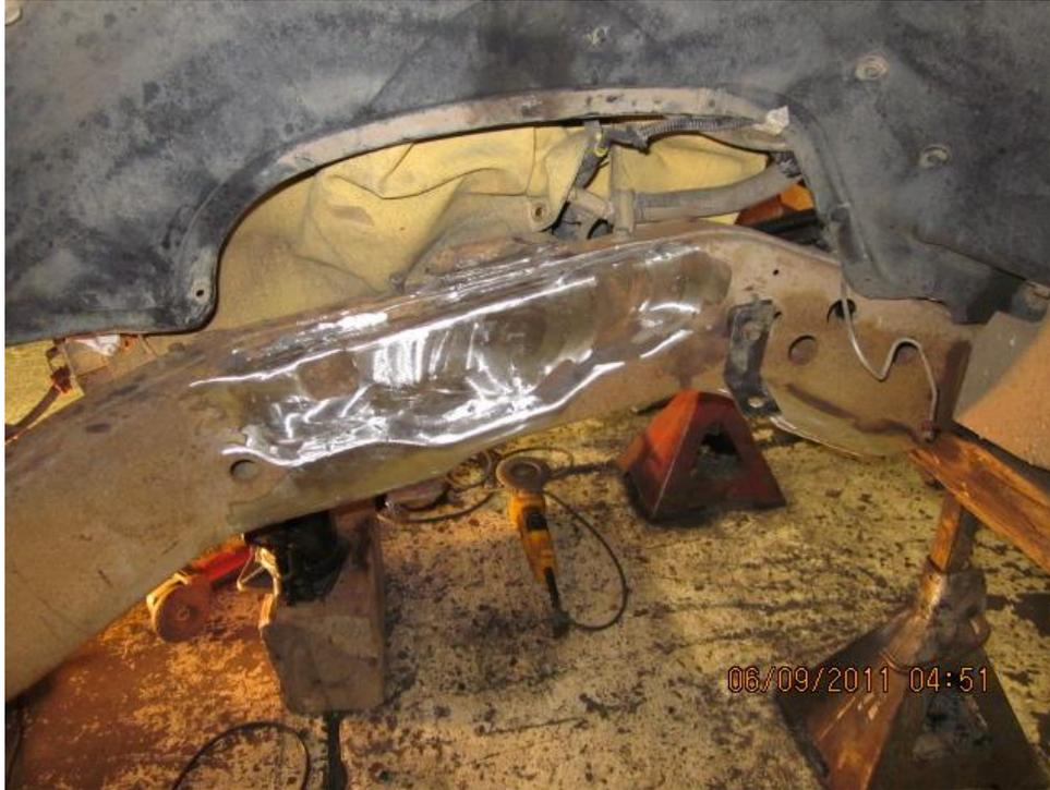
Install front hangers, additional holes will need to be drilled on the inside of each frame rail.  $\frac{1}{2}$ " x 1-1/2" bolts go in the outside of the frame rail to account for the bumper bracket,  $\frac{1}{2}$ " x 1-1/4" bolts go on the inside and  $\frac{7}{16}$ " x 1-1/4" bolts go in the bottom.
