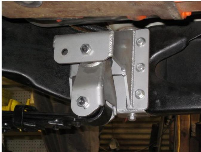
**When using stock length springs for the front of a '73-87 Chevy you will be using the front hole in these brackets**
