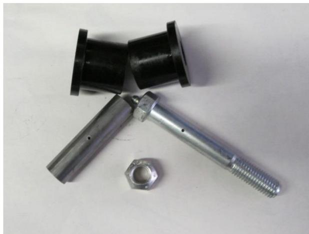
Clean the spring eye and make sure that you have removed the outer metal sleeve, all that should
