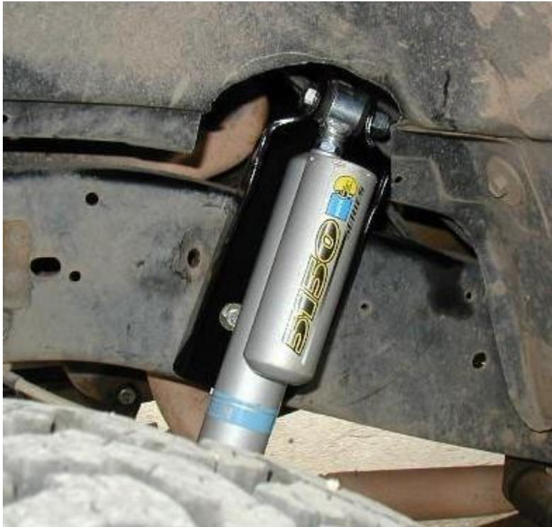
1. Remove the sheet steel half of the factory mount that's riveted to the frame with 2 rivets. You can grind the rivet heads off, use an air chisel, drill them out or even other techniques will work.
