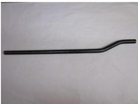
**#U9015 Draglink** - The threaded tube that links the pitman arm and steering arm. It may or may not be bent depending on application
