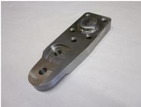
**#U9001 - RH D60 Steering arm** – The steering arm bolts to the top of your passenger side steering knuckle. It is supplied with 4 tapered nuts to attach the arm to the knuckle studs. The arms come drilled with a 5th hole in front for the extra attachment point on our Reid Racing HD knuckles. The RH arms also come with 2 tapered holes in the front so you can run the tie rod over the leaf springs using our High Steer conversion. The draglink will attach to the front hole.
