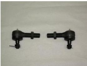
**# U9016 - Tie rod ends.** The tie rod ends screw into your draglink to attach to the steering arms and pitman arm. The same end kit is used for the High Steer tie rod. The ends should come with the jam nuts and castle nuts in the package. 1 right hand thread and 1 left hand thread.
