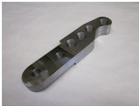
**#U9010 - RH D44 Steering arm** – The steering arm bolts to the top of your passenger side steering knuckle. The arm is drilled with a 4th hole in front for the extra attachment point on our Reid Racing HD knuckles. The RH arms also come with 2 tapered holes in the front so you can run the tie rod over the leaf springs using our High Steer conversion. The draglink will attach to the front hole.
