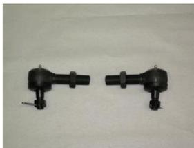
**# U9016 - Tie rod ends.** Tie rod ends that screw into your draglink to attach to the steering arms and pitman arm. The same end kit is used for the High Steer tie rod. The ends should come with the jam nuts and castle nuts in the package. 1 right hand thread and 1 left hand thread.
