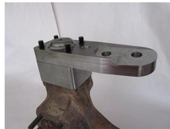
Tighten the locking nuts on top of the tapered cone adapters to 90 ft-lb and only loosen and re-tighten one time. The kingpin spring is held down by our billet riser block. Once installed and when you're greasing the zerk in the steering arm, grease will fill the cavity in the steering arm first then flow through the hole in the top of the riser block into the upper kingpin parts.
