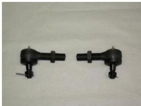
**# U9016 - Tie rod ends.** The tie rod ends screw into your draglink to attach to the steering arms and pitman arm. The same end kit is used for the High Steer tie rod. The ends should come with the jam nuts and castle nuts in the package. 1 right hand thread and 1 left hand thread.
