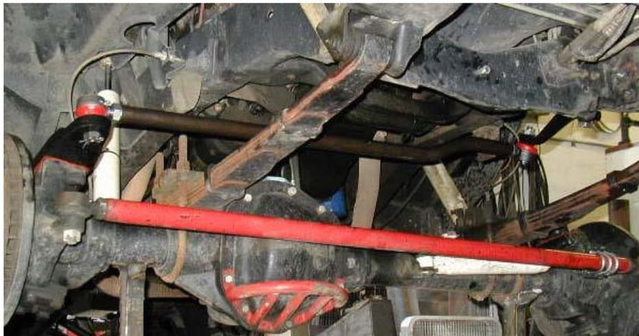
Be sure to check the fastener torque after a test drive and verify after any hard trail use.
