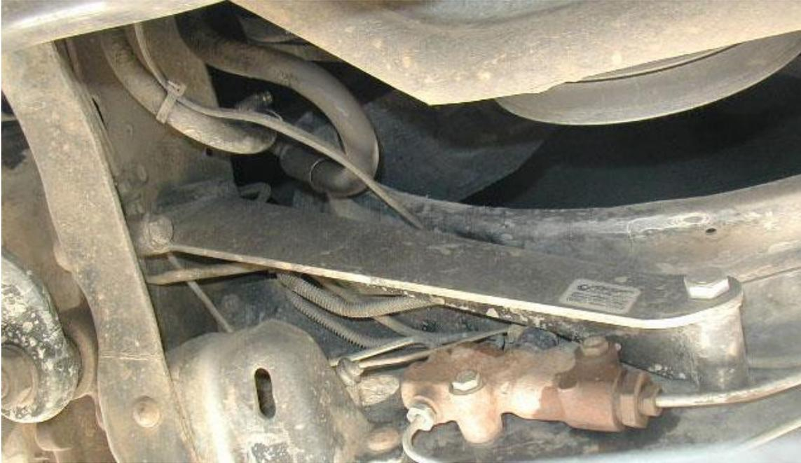
4. Mark the crossmember by pushing a marker or punch through the end of the steering box brace. Remove the larger steering box brace from the truck.
