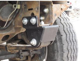
Position rear hanger such that the distance from the main eye centerline to the upper shackle bolt is 46.5". You will be using the forward most shackle bolt location, the bent piece of the bracket goes towards the front of the truck.
